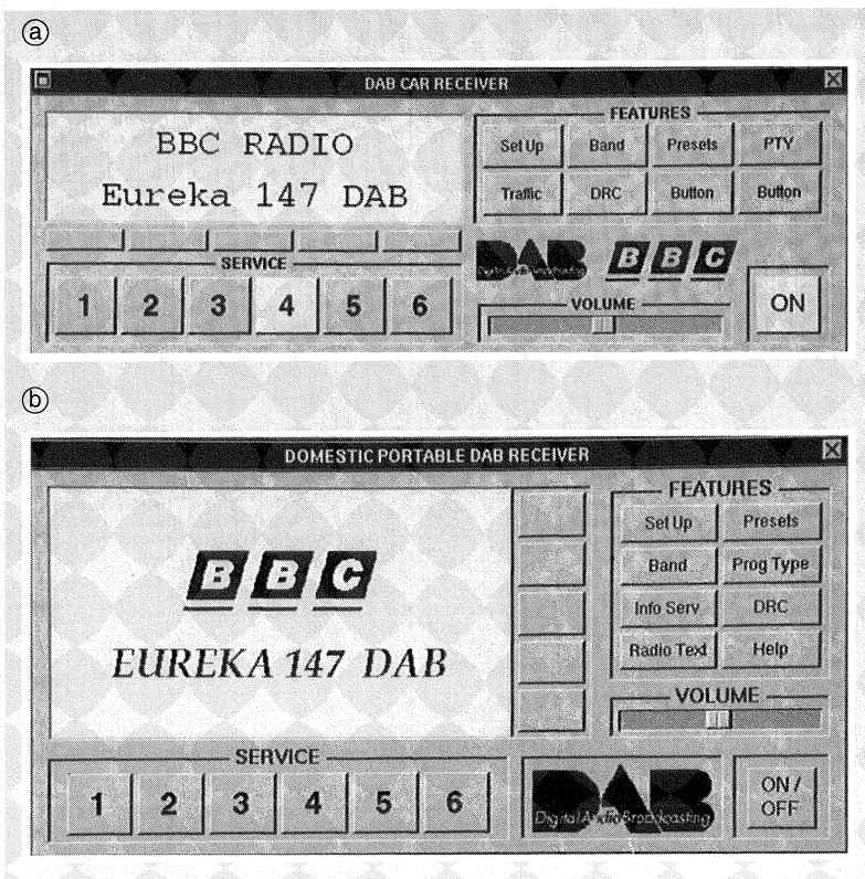
Figure 7 Simulated DAB receiver front panels: a) Car receiver b) Home receiver.
